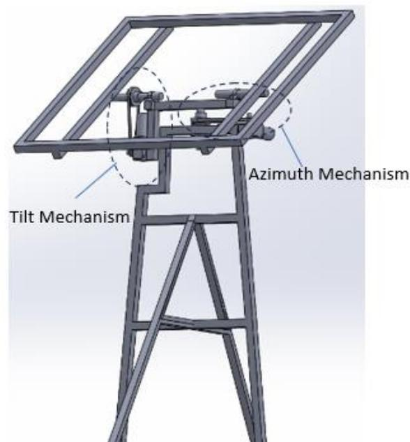
Fig. 1. The concept of rig of STS system
