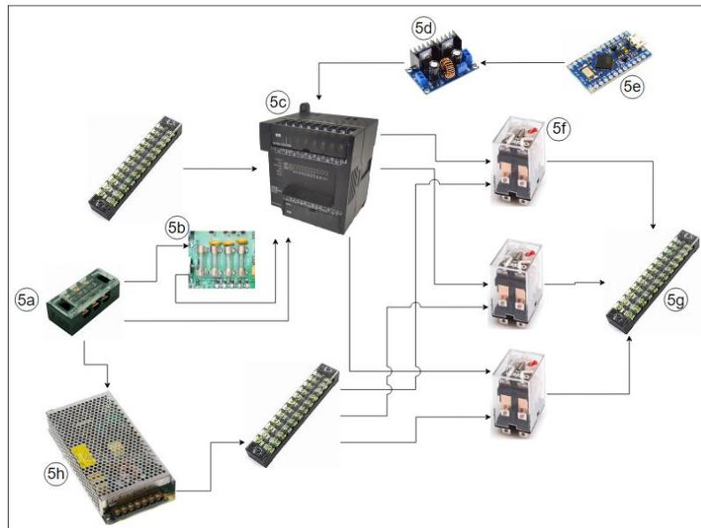
Fig 2. Soil moisture controller concept schematic
