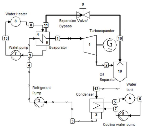
Fig. 1. Organic Rankine cycle: experimental setup (left), schematic setup (right)
