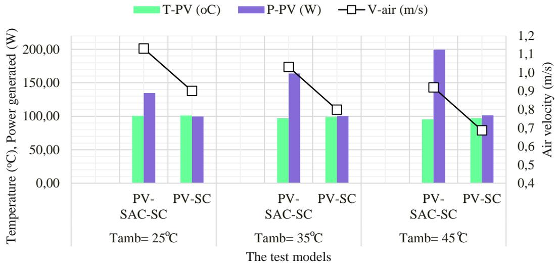
Fig. 1. The relationship between the temperature of the PV modules, the power, and the airflow velocity inside the SC at the three Tamb: 25 °C, 35 °C, and 45 °C
