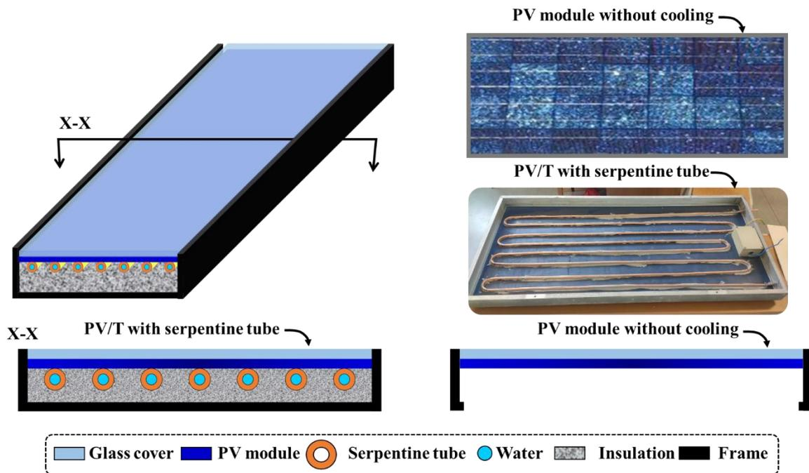
This experiment aims to assess the performance of a presented module of the water-cooled PV/T by improving the heat extraction through a serpentine tube mounted to the PV module to decrease the cell temperature, which effectively enhances the productivity of the PV/T modules.
