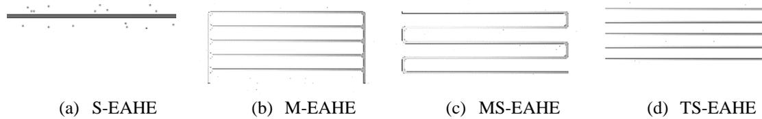
Fig. 1. The four EAHE configurations.
