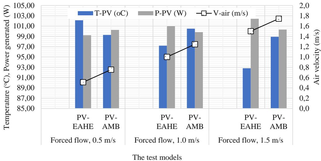
Fig. 1. The relationship between the temperature of the PV modules, the power, and the airflow velocity inside the SC at the three air fan forced speeds: 0.5 m/s, 1.0 m/s, and 1.5 m/s.
