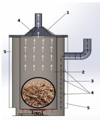
Fig. 1. Pyrolysis Reactor Schematic
