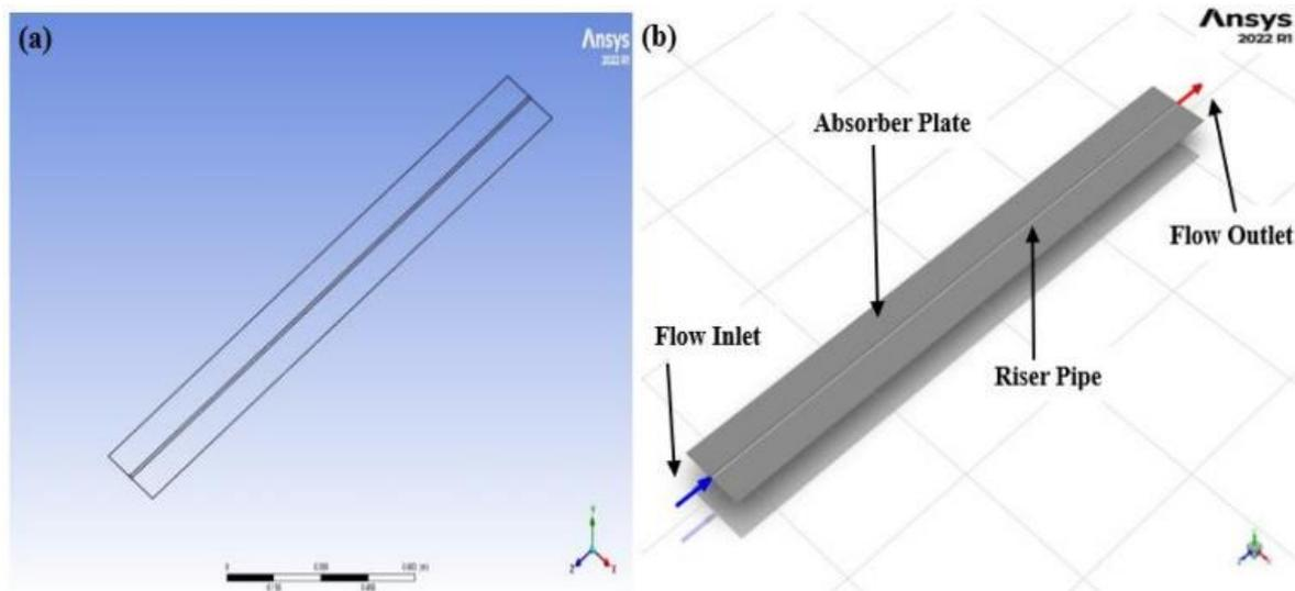
Fig. 1. Model geometry of the computational domain of FPSC: (a) Isometric wireframe view and (b) 3D design
