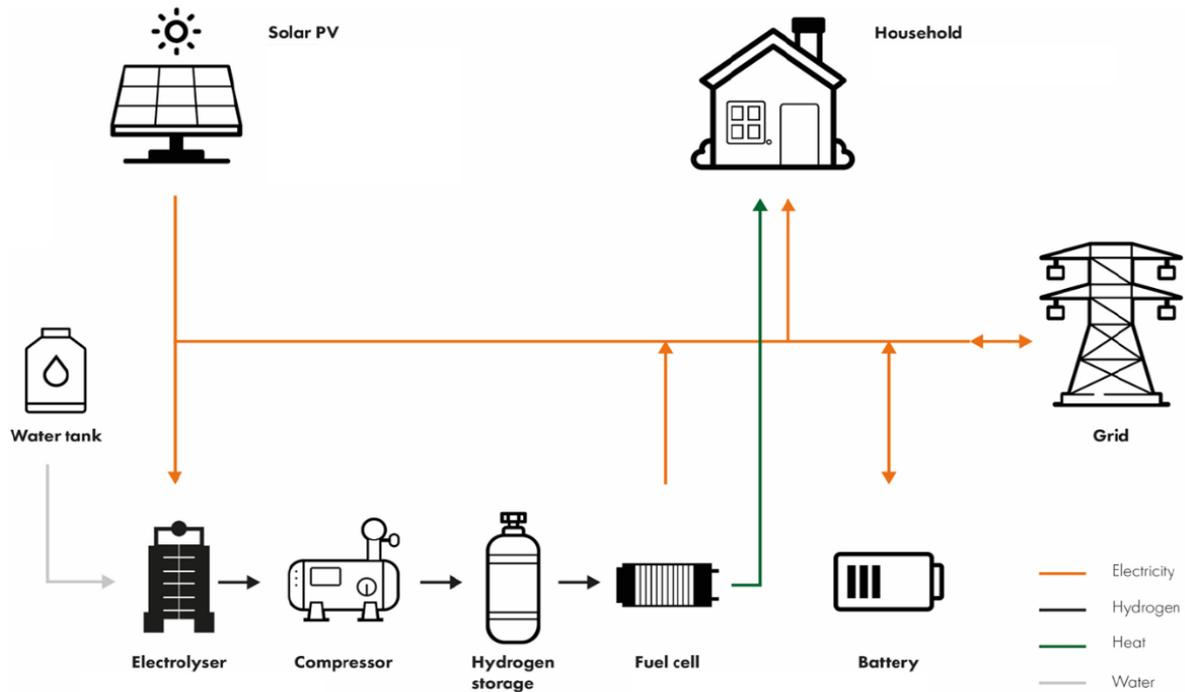
Fig. 1. System components of a household H<sub>2</sub> based storage system
