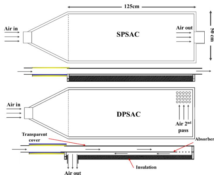
Fig. 1. Schematic view of the test rigs
