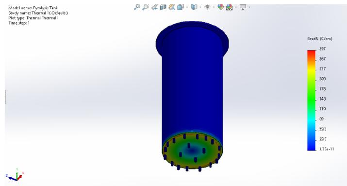
Fig. 2. Reactor Temperature Simulation
