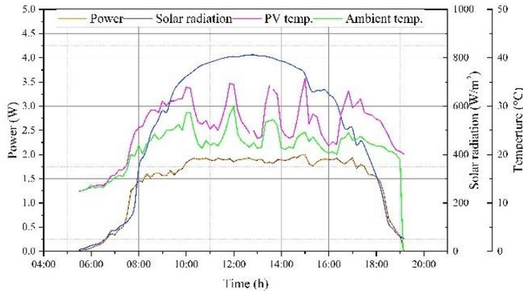
Fig. 1. The power generation from spherical PV module
