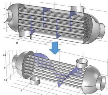
Fig. 1. Illustration of segmental baffles to helical baffle
