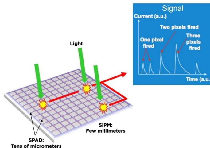
The silicon photomultipliers have several advantageous characteristics, including high photon detection efficiency (PDE), good single photon time resolution (SPTR), high gain that
