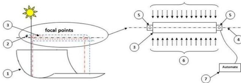
Fig. 1. Components of a cylindro-parabolic concentrator (CPC)
