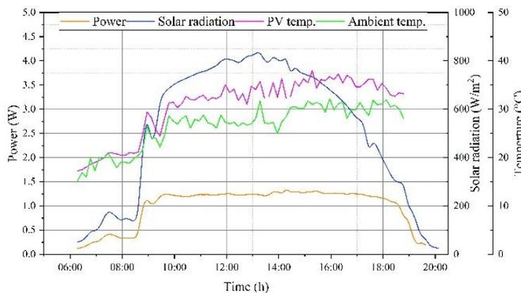
Fig. 2. The power generation from hemispherical PV module
