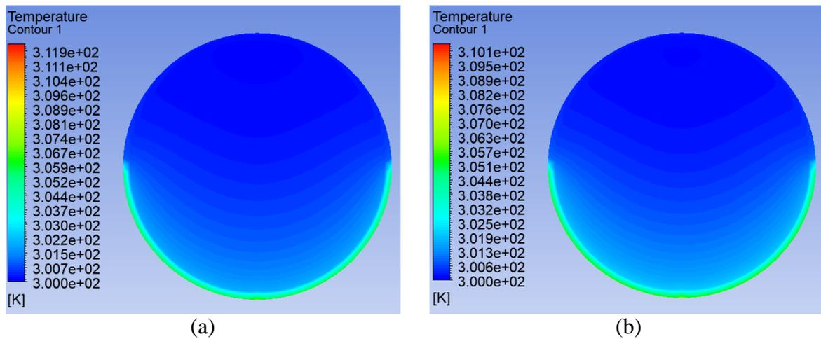
Fig. 1. Temperature countours: a) water, b) nanofluid
