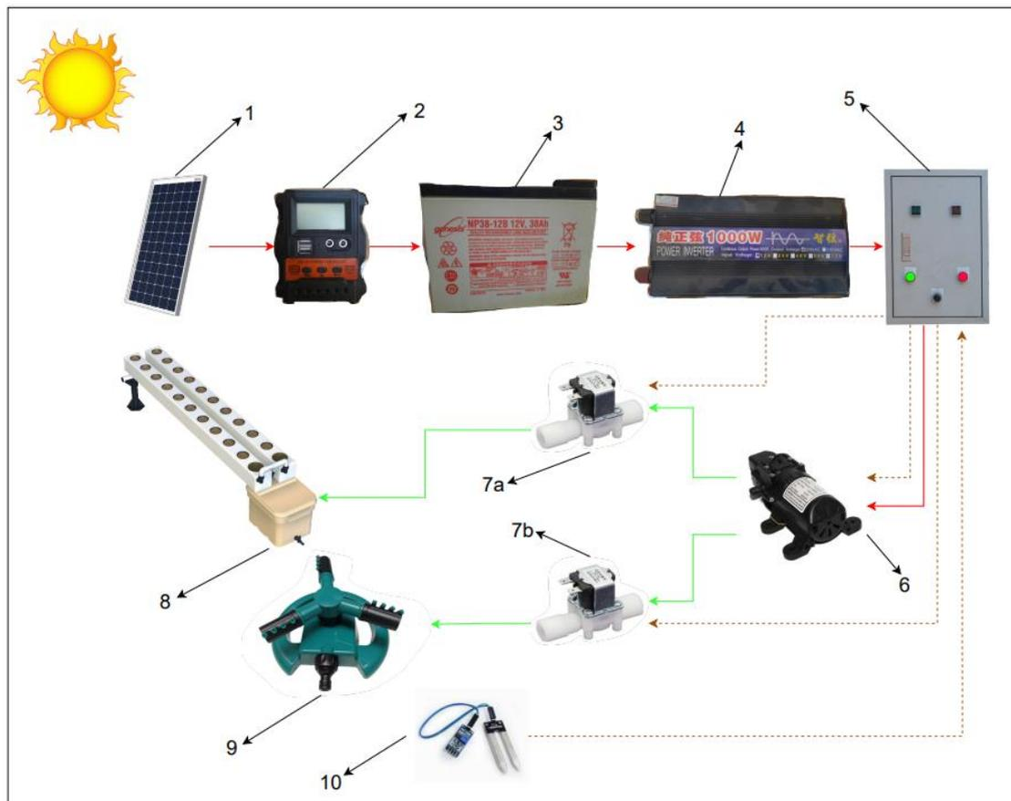
Fig. 1. The concept of agrivoltaic components
