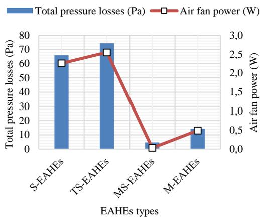
Fig. 2. The total pressure losses and the air fan power of the four EAHE types.
