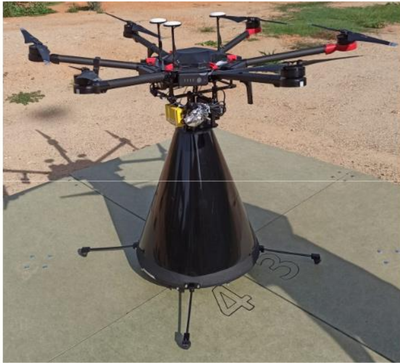
Figure 7. Radioluminescence detection system integrated with the DJI Matrice 600 Pro and ready to fly.
