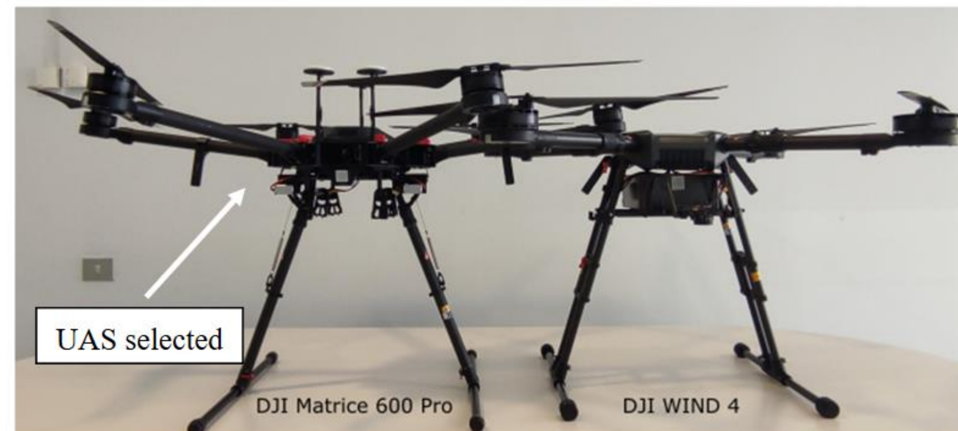
Figure 5. Unmanned Aircraft System candidates for mounting the alpha detector system.
